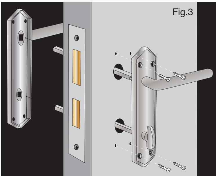
1 -Locate the spindle through the square hole in the bathroom lock and attach the backplates onto the spindle on each side of the door.
