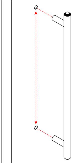
1. Drill holes to the appropriate size, in the position required and counter sink.
