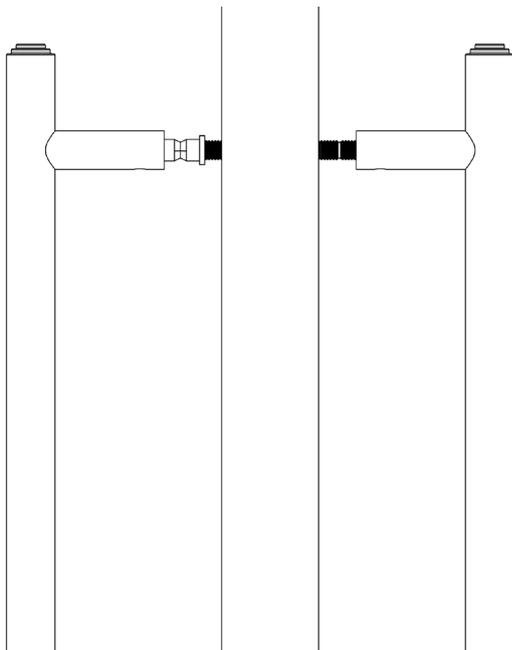
3. Place the other pull handle on the opposite side of the door, over the brass head of the bolt. You may need to loosen the grub screws first.
