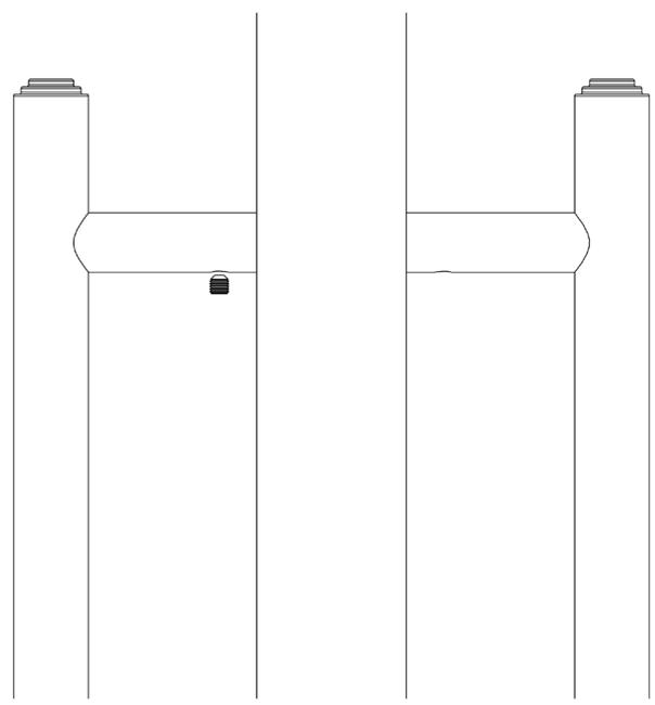
4. Now the pull handle is in the back to back position, tighten the grub screw top and bottom to the brass head.
