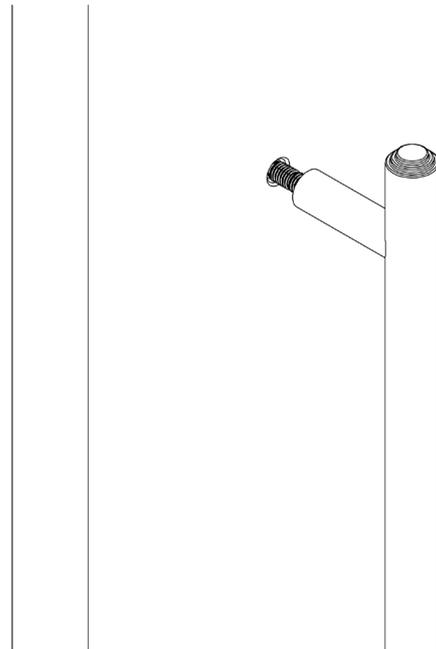
2. Push the back to back bolts through the newly drilled holes, and screw into the pull handle.
