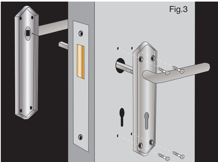
1 -Locate the spindle through the square hole in the lock and attach the backplates onto the spindle on each side of the door.
